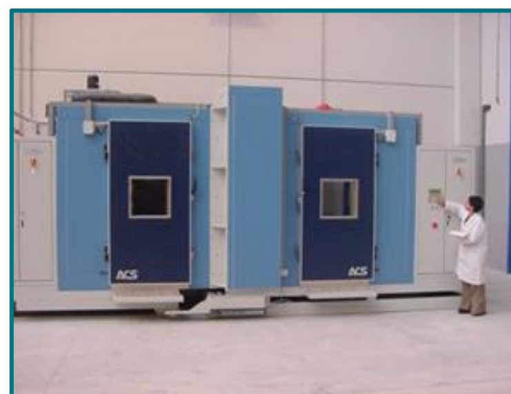
Guarded hot box test
