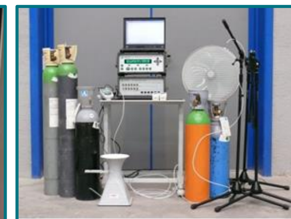
Tracer gas leak test
