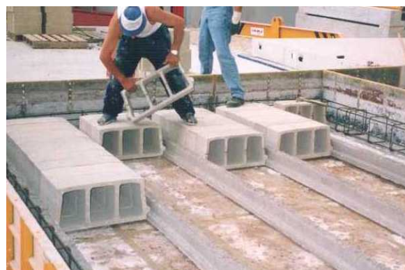
Fig. 1. Beam and block floor mounted in laboratory.
